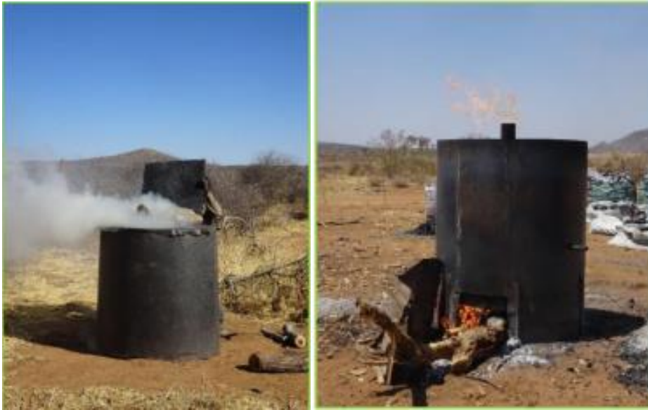
Figure 9 Namibian traditional drum (left) and retort kiln (right) (Temmermann 2016)
